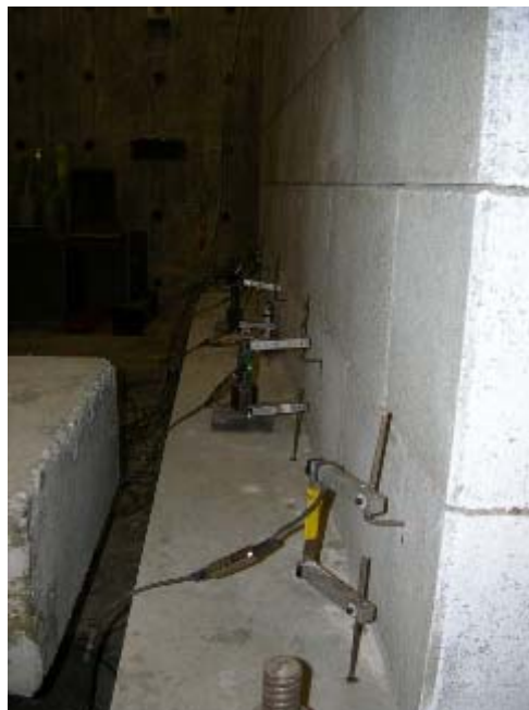
Figure 5-3 Instrumentation used to measure uplift at the base of the wall
