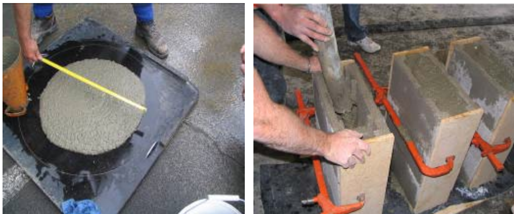
Figure 3-1 Spread test of Formfill and construction of prisms for testing
