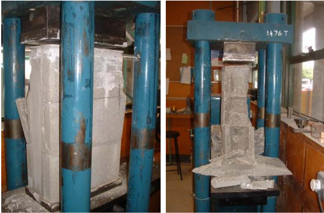
Figure 3-3 Failure mechanism of Set 2 prisms
