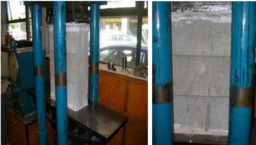
Figure 3-2 Test set-up of masonry prisms
